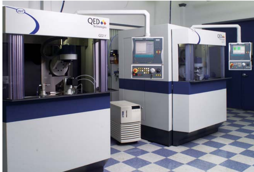
Figure 2. The Q22-Y MRF system is QED's flagship machine, enabling the manufacture of precision optics while reducing overall production time, increasing yield and reducing costs.
