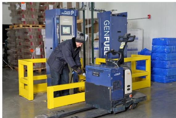
An operator adds hydrogen to his fuel cell-powered pallet jack
